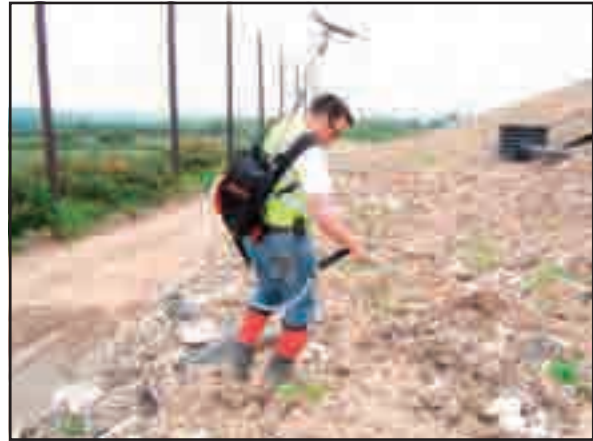
Figure 8.7 Monitoring of surface emissions from the flank of a landfill cell
