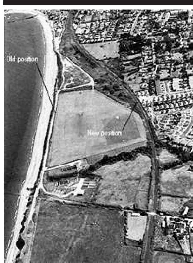
Figure 7. Coastal squeeze and buffering. Realignment inland of the railway at Greystones, County Wicklow, showing the old and new track positions (NCEC, 1992).
