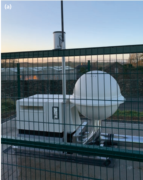
Figure 14.10 (a) A high-volume air sampler in the National Radiation Monitoring Network, and (b) a gamma spectroscopic measuring system in the upgraded National Radiation Monitoring Network
