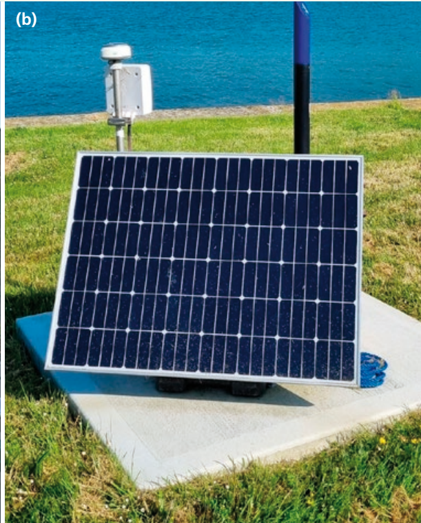
Figure 14.10 (a) A high-volume air sampler in the National Radiation Monitoring Network, and (b) a gamma spectroscopic measuring system in the upgraded National Radiation Monitoring Network
