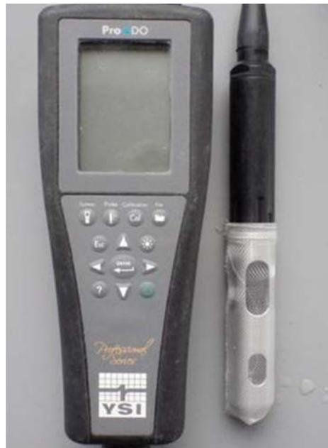
Figure 2 YSI Luminescence Oxygen Meter
