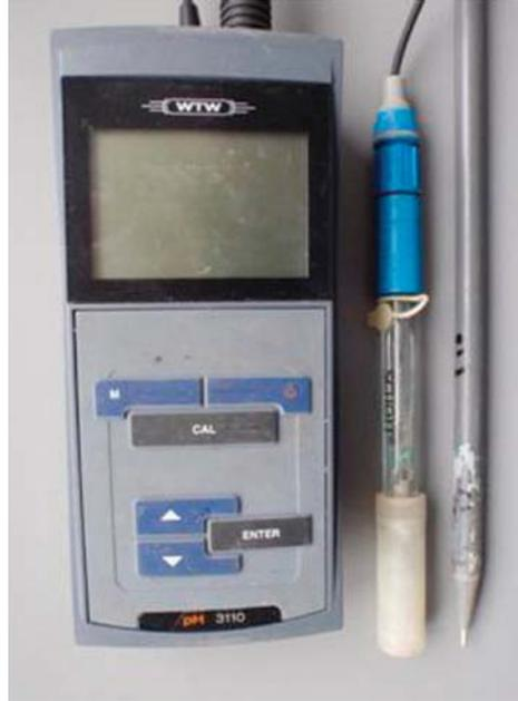
Figure 3 WTW Redox Potential Meter
