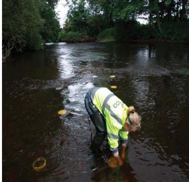
**Figure 5 Setting Sediment Traps in River Nore**
