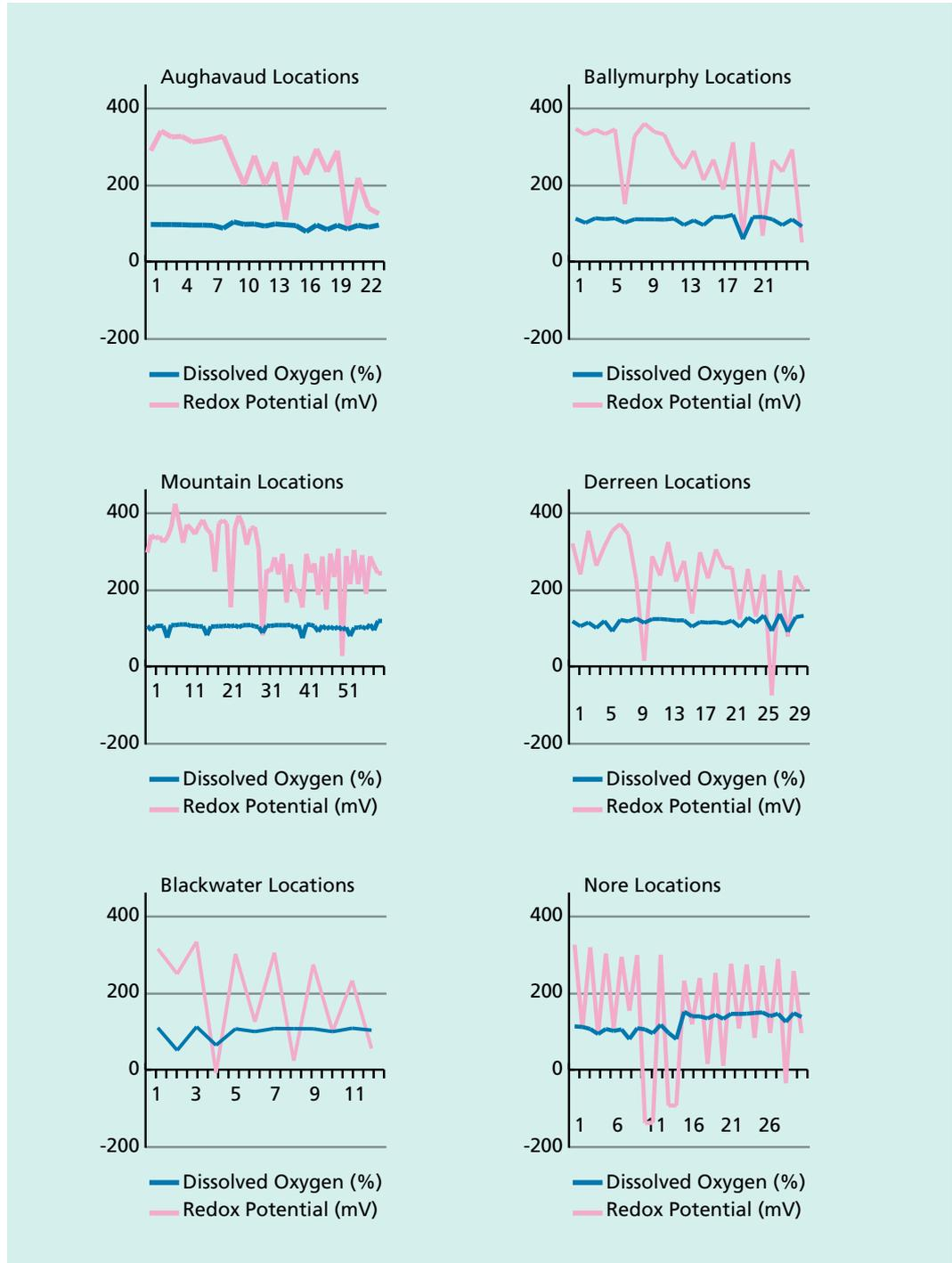
Figure 19 Redox (mV) and dissolved oxygen (% saturation) measurements in water at locations on six rivers. Some measurements were repeated at same sites, e.g. Mountain River
