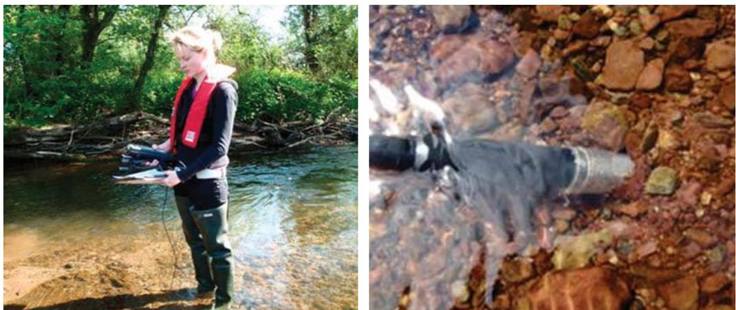
**Figure 17 Showing measurement of dissolved oxygen (Detail – probe at 5cm in river substratum)**
