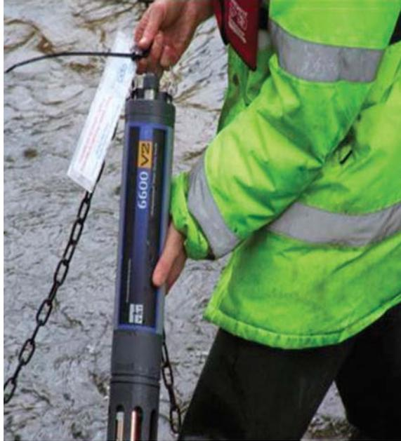
Figure 4 Sonde Water Quality Data Logger
