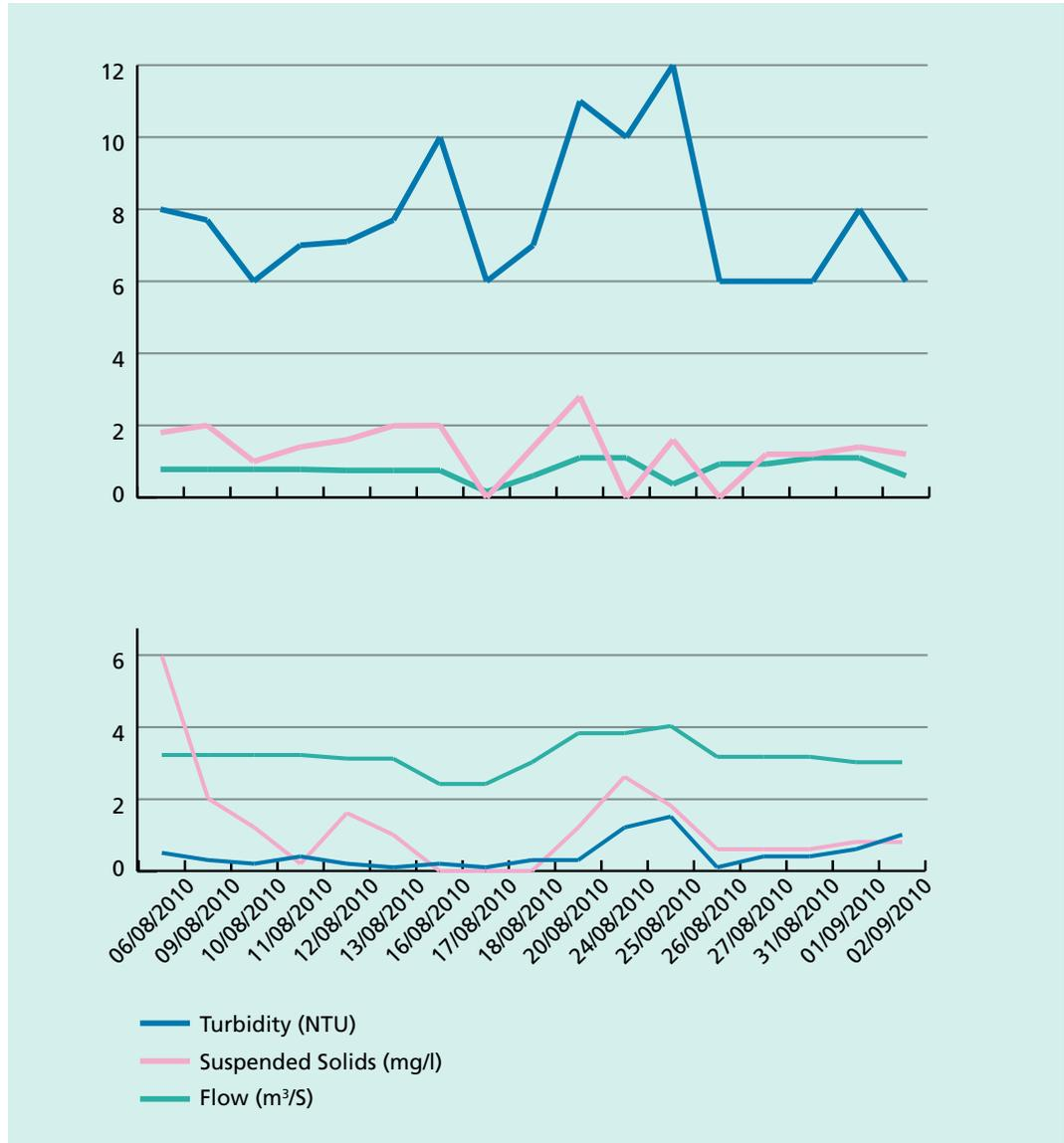
Figure 11 Showing measurements of turbidity (NTU) and suspended solids (mg/l) at Kilbricken (above) and Ballyragget (below) during period of relatively stable river flow (m³/s)
