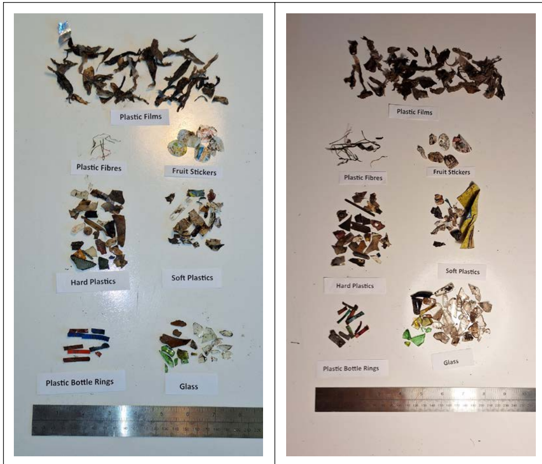
Figure 2.2. Photograph of the visible contamination found in two different 15L compost samples.
