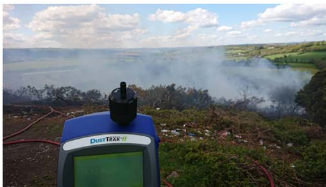
Figure 5.5. Sampling PM 2.5 in smoke in Cobh, Co. Cork (left), and near Killarney, Co. Kerry (right). Photographs: Clara Felberbauer.
