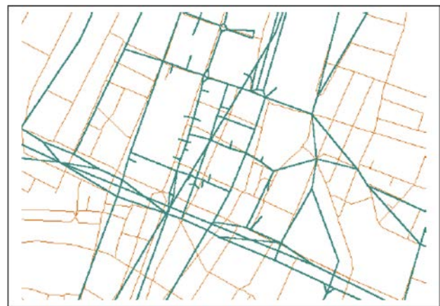
Figure 3.1. An example of an accurate digital road network model (brown) and an inaccurate road traffic network model (green). Source: based on WG-AEN (2007, p. 19).
