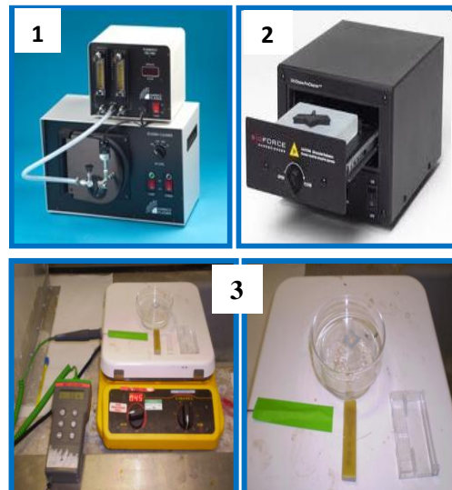
Figure 25 Common bonding techniques: (1) oxygen plasma activation; (2) UV bonding and (3) solvent bonding using hexane.
