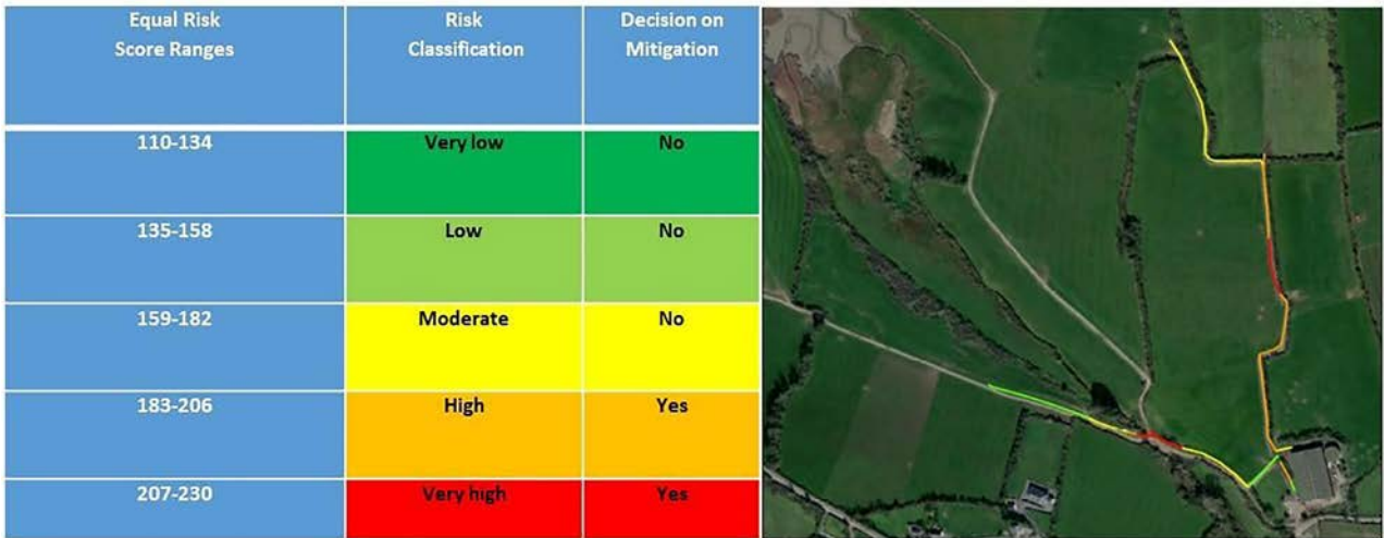
Figure 3.5. An example showing the risk classification, decisions on the need for mitigation and an output map for a given farm roadway section developed within the project. Adapted from Rice et al. (2022); licensed under CC BY 4.0 ( https://creativecommons.org/licenses/by/4.0/ ).
