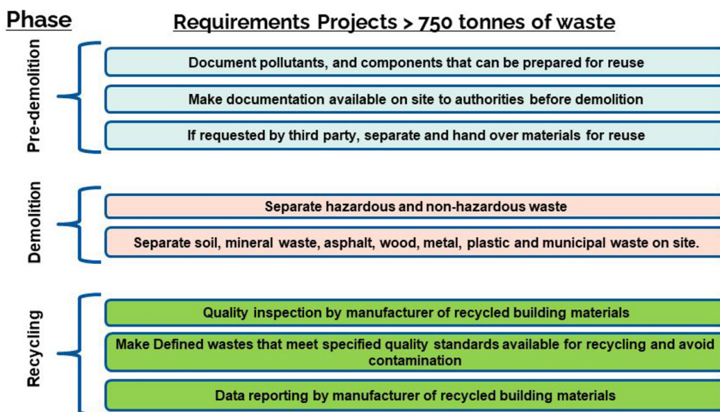
Figure 4.30. Austria's Recycling Building Materials Ordinance.
