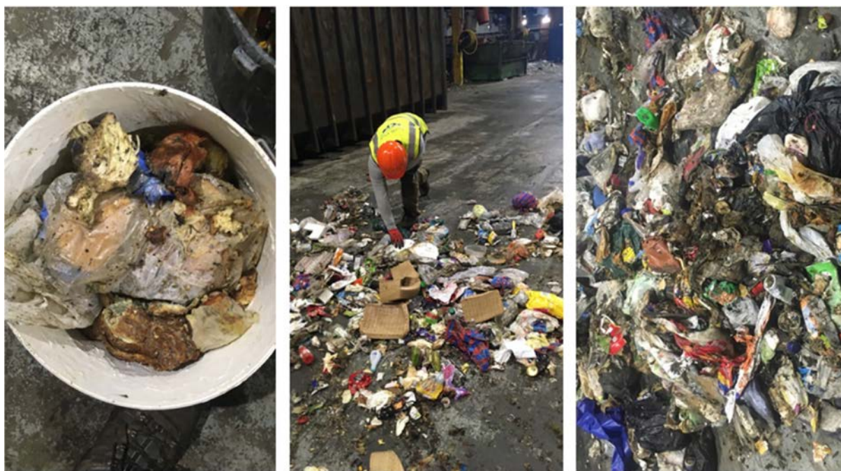
Figure 5.1. Measuring the food waste content of the general waste stream in Ennis in May 2022.
