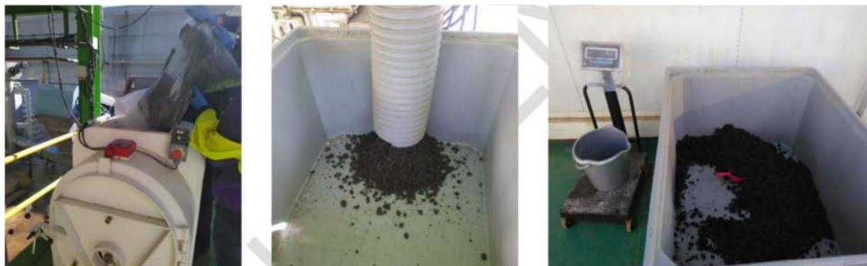
Figure 6.1. Pre-treatment (milling and homogenisation) of the MS-OFMSW prior to fermentation.
