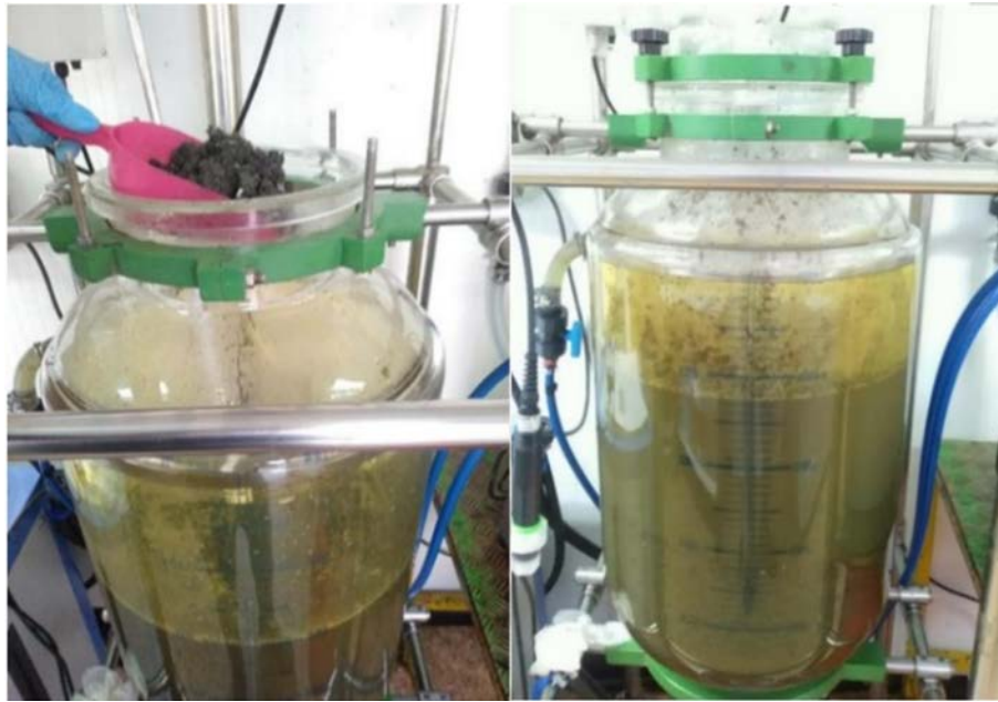
Figure 6.2. Loading of the pilot reactor (left) and the resulting homogeneous aqueous organic mixture (right).
