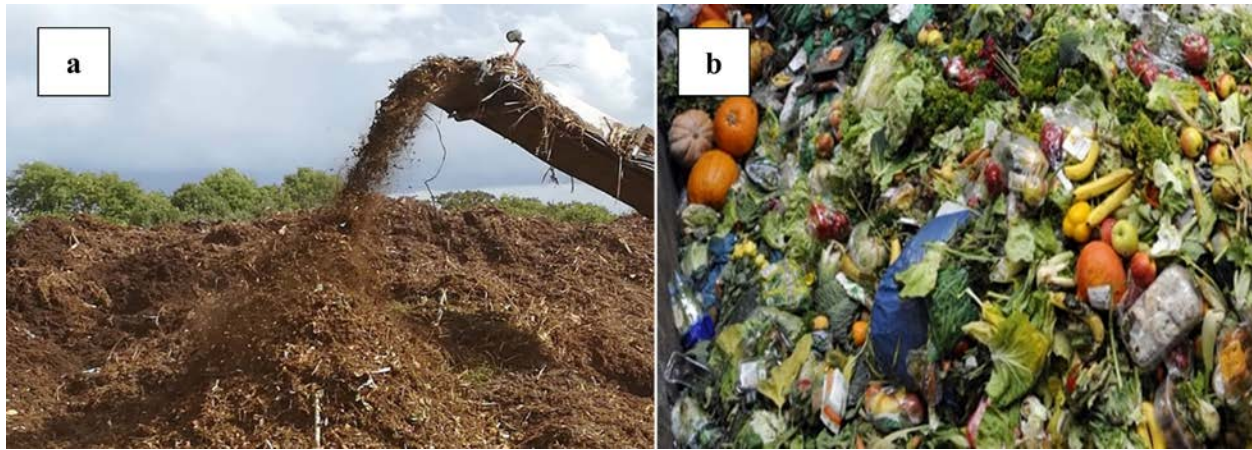
Figure 9.1. (a) Shredding of source-segregated green waste at processing facility and (b) source-segregated food waste.
