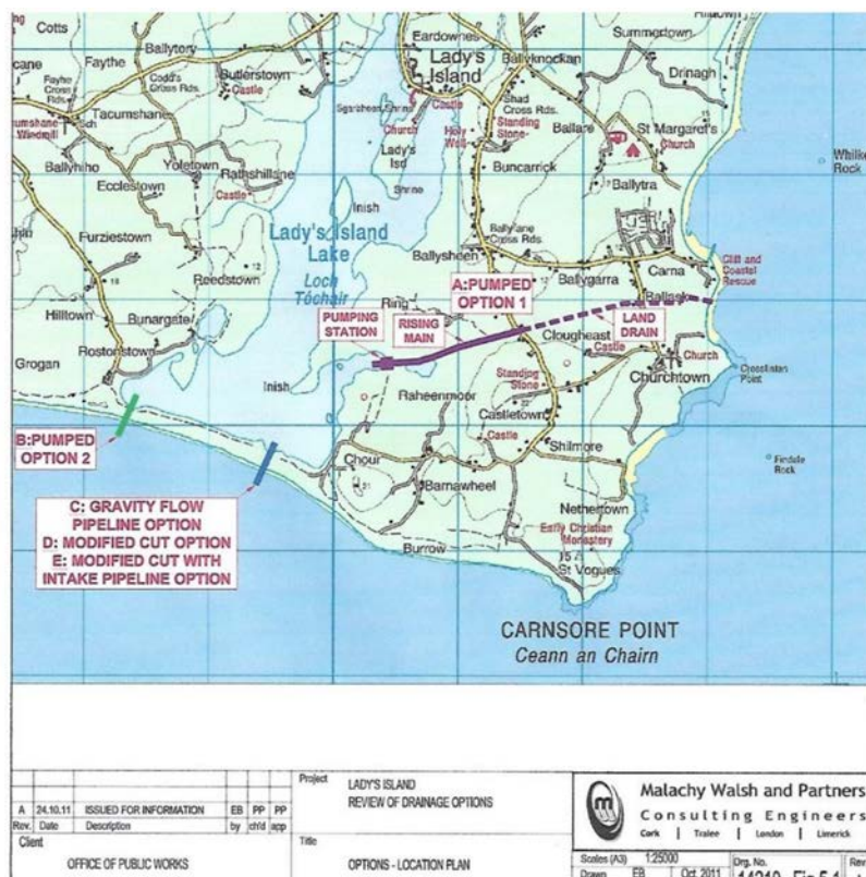
Figure 5.1. Map of Lady's Island Lake showing possible solutions for controlling water levels. Reproduced with kind permission of Malachy Walsh.
