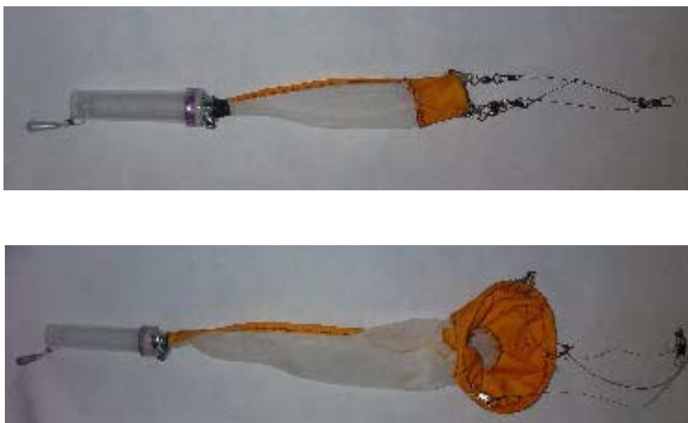
Figure 2.2. Net samplers for boreholes (top) and wells (bottom).
