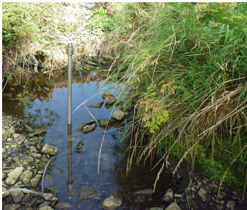
Figure 2.3. Hyporheic sampling pipe in a Burren stream.
